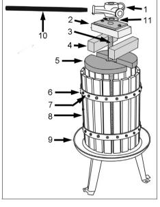
the pressure plate (2) on top of these, as shown in the illustration. Place a container beneath the outlet spout in the base (9) ready to collect the juice.
